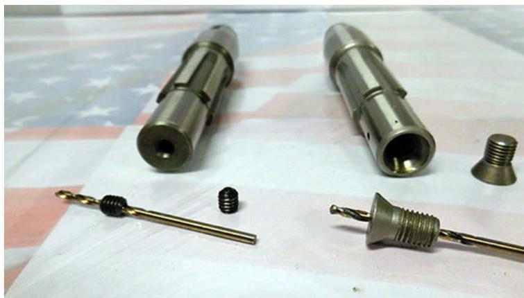
The last step in the way we achieve 360° Oiling is to plug the relief hole Harley drilled in 1938 and later cam covers.
